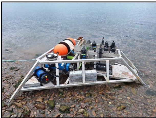
Figure 6: FAST-2 platform equipped with five Innovasea acoustic receiver technologies (with duplicates for redundancy), an ADCP and hydrophone for recording flow speed and underwater noise.
